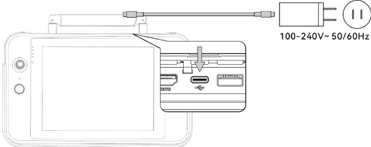
**Fig 4-9** Use the remote controller charger to charge the remote controller
