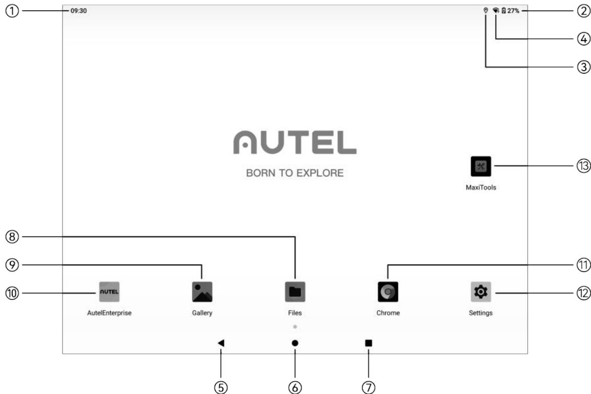
Fig 4-11 Remote Controller Main Interface
