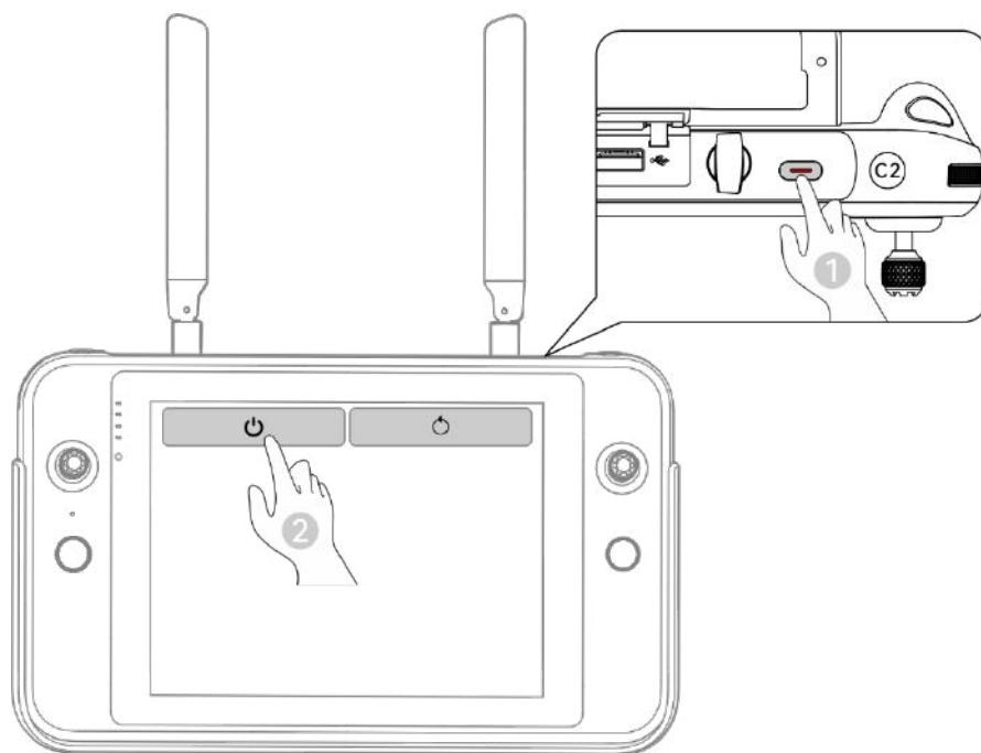
**Fig 4-7** Turning the Remote Controller Off
