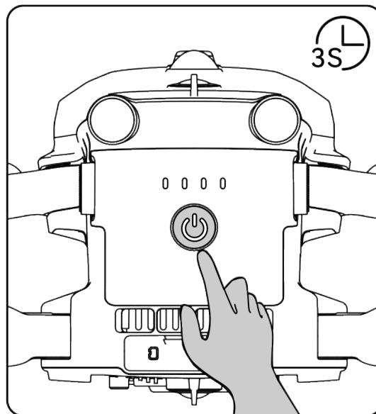
Fig 5-3 Turn On or Off the Smart Battery
