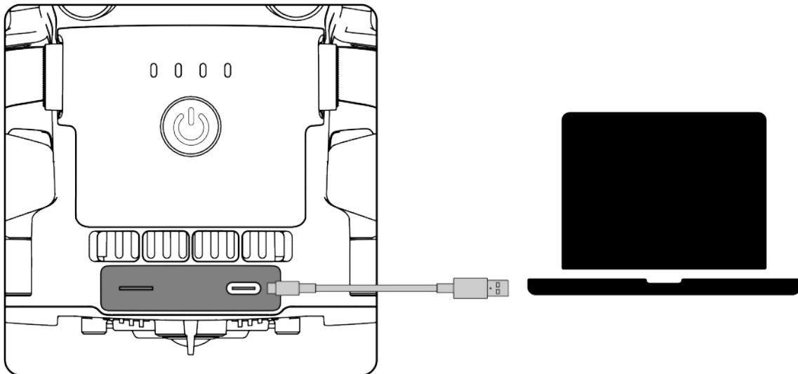
Fig 3-16 Connect to PC/MAC via Drone USB-C Port
