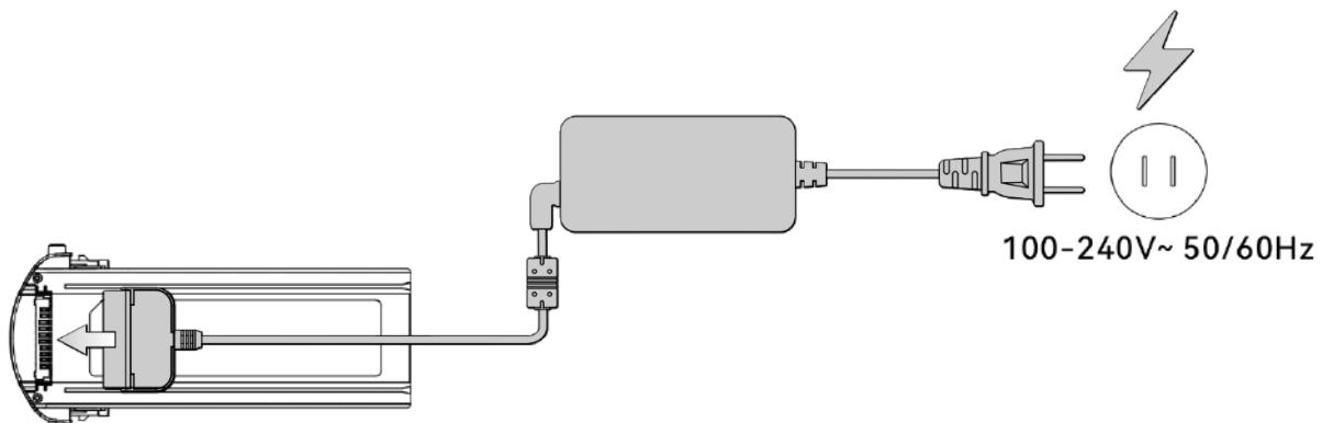
**Fig 5-7** Use the Battery Charger to Charge the Smart Battery
