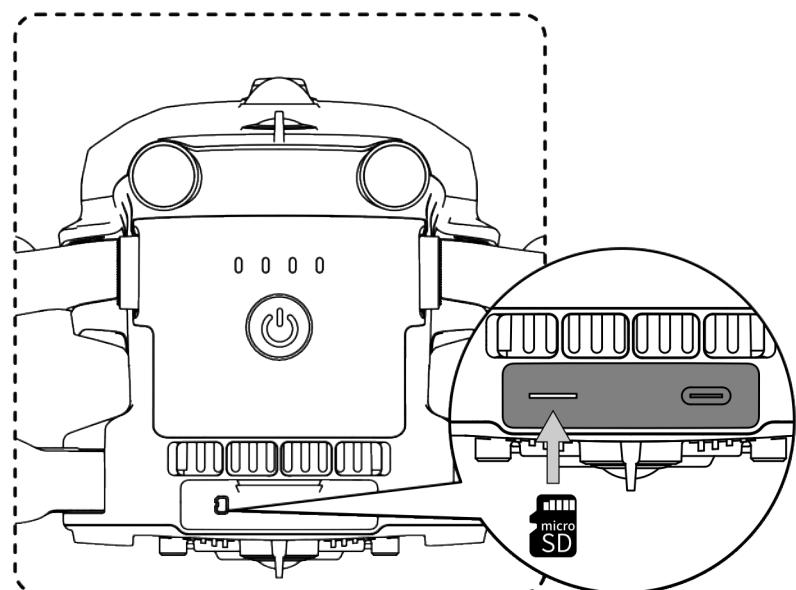
Fig 3-15 Installing the microSD Card
