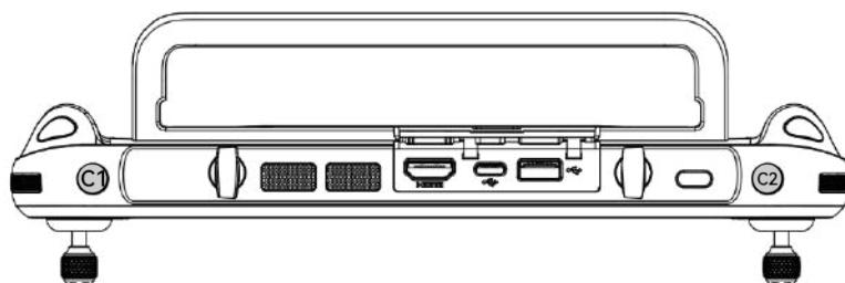
Fig 4-16 Custom Keys C1 and C2
