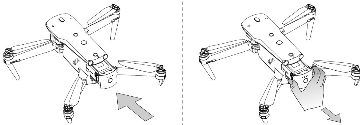
Fig 5-2 Install/Remove the Smart Battery
