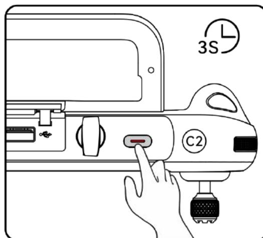
Fig 4-6 Turning the Remote Controller On
