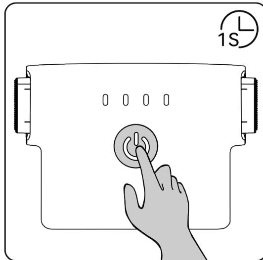
**Fig 5-4** Checking Battery Level When the Smart Battery is Off
