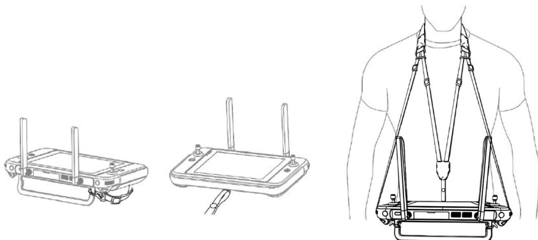
Fig 4-4 Install the Remote Controller Lanyard (As Required)
