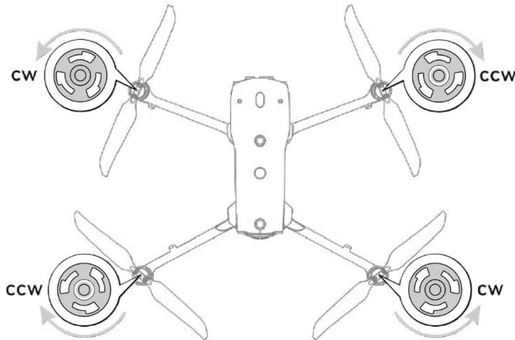
**Fig 3-5** Install the Propellers
