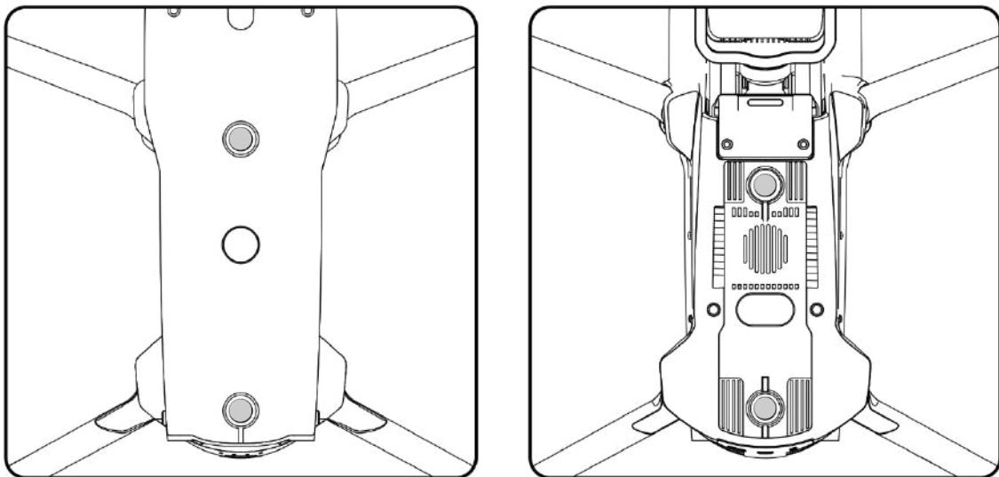
Fig 2-3 Top and bottom visual obstacle avoidance lens modules of the drone
