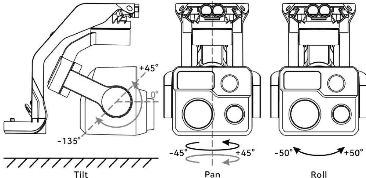
Fig 3-12 Three-axis description of the Gimbal (Fusion 4T Gimbal)
