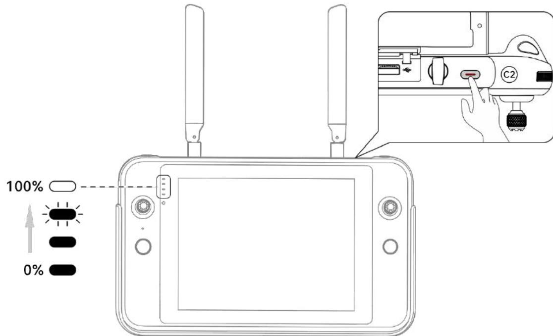
**Fig 4-8** Checking the Battery Level of the Remote Controller
