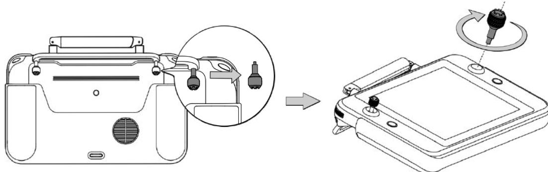
Fig 4-5 Installing sticks
