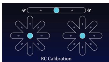
3. Push both **Command Sticks** to the ends of their 8 directions, and turn the **Gimbal Pitch Dial** clockwise and counterclockwise to its 2 ends, holding respectively until you hear a beep.
