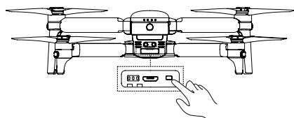
3. Press and hold the **RC Pairing Button** for about 3 seconds, the **Pairing Indicator** will flash quickly indicating the aircraft is ready to pair with the remote controller.
