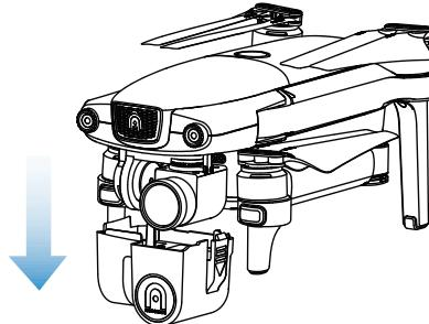
Reinstall the gimbal holder after using the aircraft to protect the gimbal from accidental damage when not in use.
