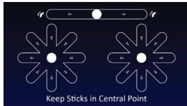
2. Release both **Command Sticks** and the **Gimbal Pitch Dial** naturally to the central position. The three central rounds on the RC calibration screen will be highlighted successively.
