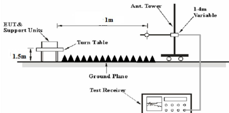
The radiated emission Below 1GHz tests were performed in the 3 meters chamber test site A , above 1GHz tests were performed in the 3 meters chamber test site A, using the setup accordance with the ANSI C63.10-2013. The specification used was the FCC 15.209, and FCC 15.407 limits and RSS-247, RSS-Gen limits.
