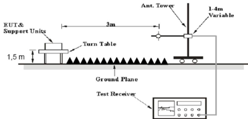
The radiated emissions were performed in the 3 meters distance, using the setup accordance with the ANSI C63.10-2013. The specification used was the FCC 15.209, and FCC 15.247, RSS-247,RSS-Gen limits.
