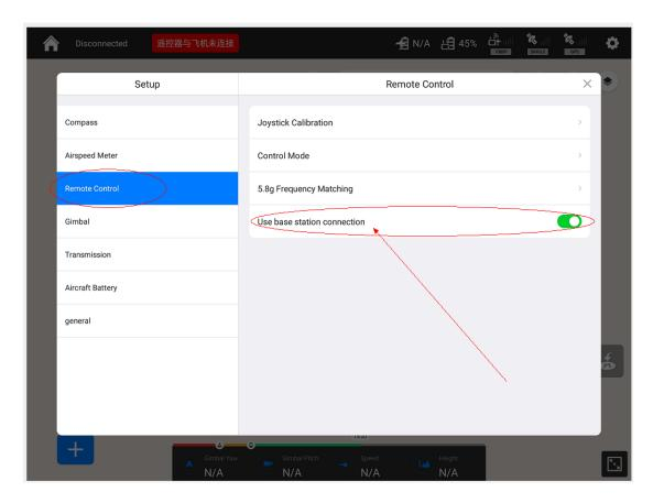
When connect the UAV through base station, follow the up steps to setup.
