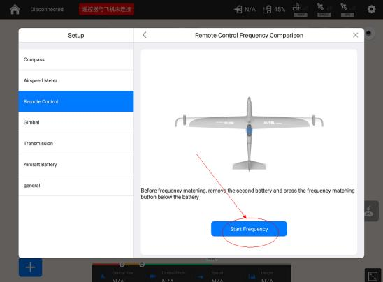
When connect the UAV direct, and match the RF connection, setup the up steps.
