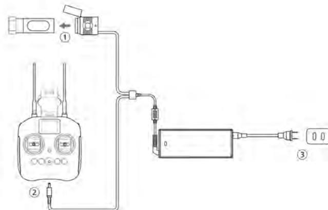
1. Remove the battery from the aircraft and connect it to the charger.
