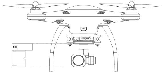
Reinstall the gimbal holder after using the aircraft to protect the gimbal from unwanted movements when not in use.
