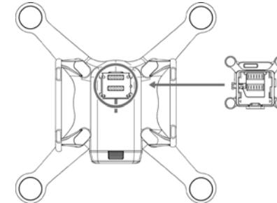
2. Slide the **Quick-mount Module** onto the **Quick-mount Base** towards the **Lock** direction (
