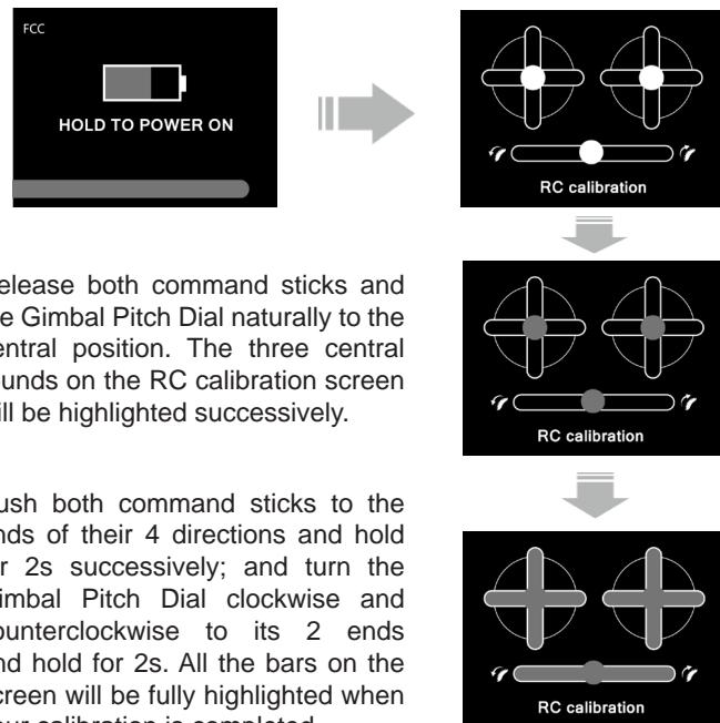
2. Release both command sticks and the Gimbal Pitch Dial naturally to the central position. The three central rounds on the RC calibration screen will be highlighted successively.
