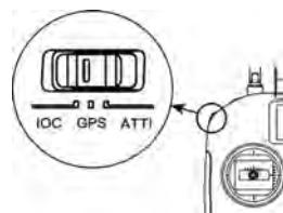
IOC mode is also known as Carefree Mode. It is used to keep the aircraft's direction controls locked regardless of its nose direction. It is most useful when you are unable to observe the nose direction of the aircraft. IOC works only in GPS mode, and has 2 control modes: **Home Lock** and **Course Lock**.
