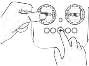
4. Push and hold the **Left Command Stick** leftward while pressing and holding the **Power** button on the remote controller for a few seconds, the binding indicator will turn to solid green light when binding is successful.
