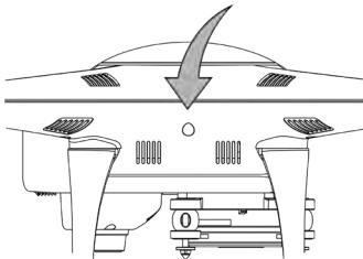
3. Press and hold the **RC Binding button** on the aircraft for about 3 seconds, the binding indicator beside the **RC Binding button** will flash slowly in green light indicating the aircraft is ready to rebind.
