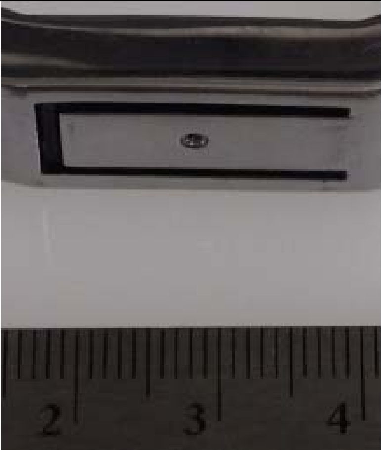
Close up of Antenna Embedded into Bracelet Frame
