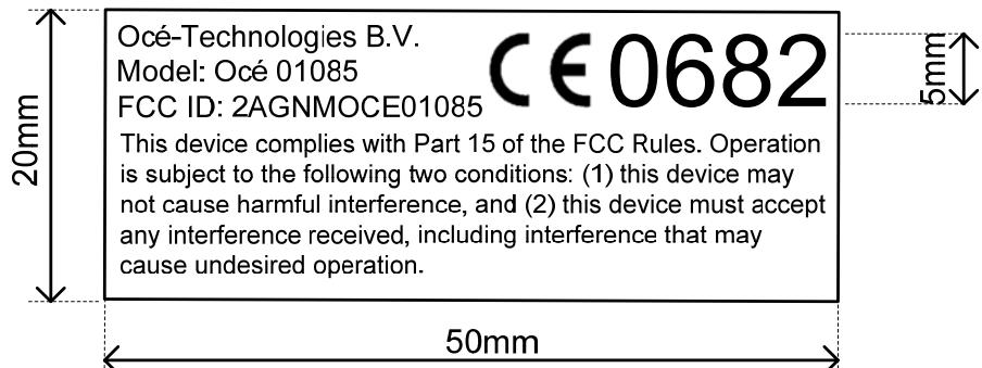
The label is located at the backside of the enclosure:
