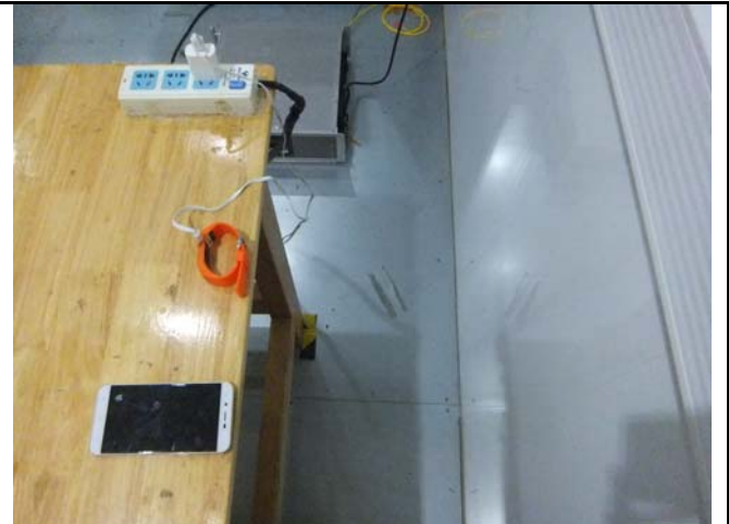
Conducted Emissions Test Setup Side View
