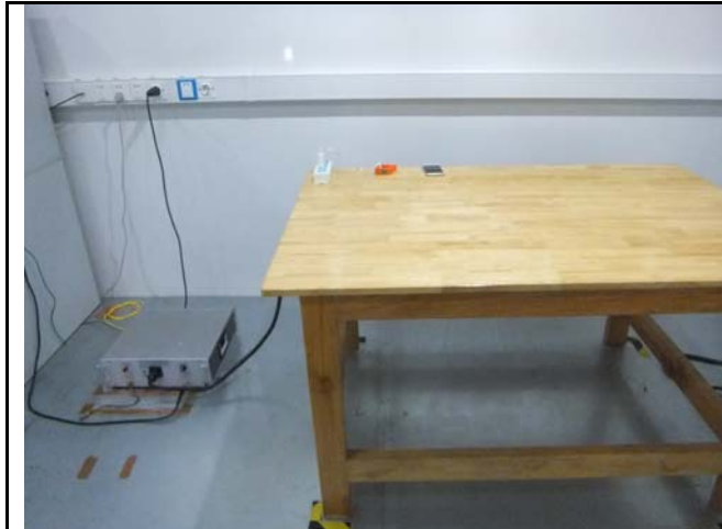
Conducted Emissions Test Setup Front View
