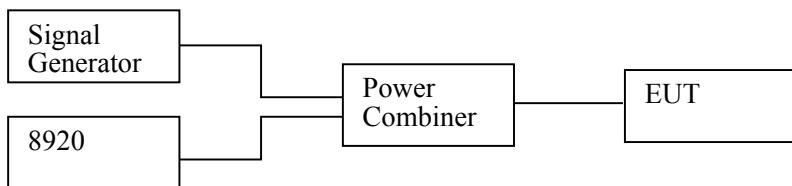
2. Apply a signal to the EUT antenna port at lowest, middle, highest channel frequencies of the operating band;
