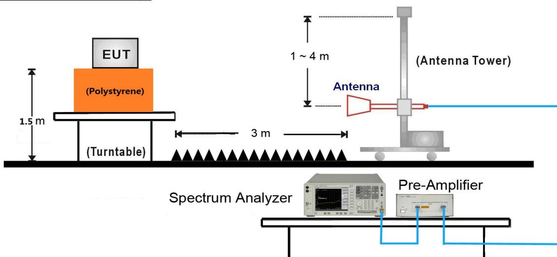
18GHz ~25GHz Test Setup:
