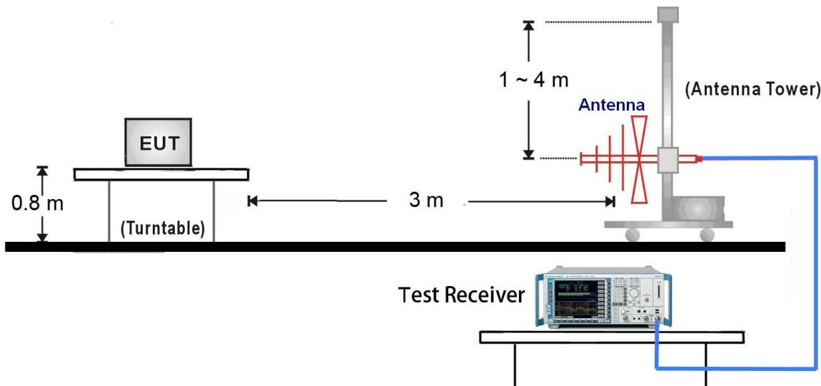
1GHz ~ 18GHz Test Setup:
