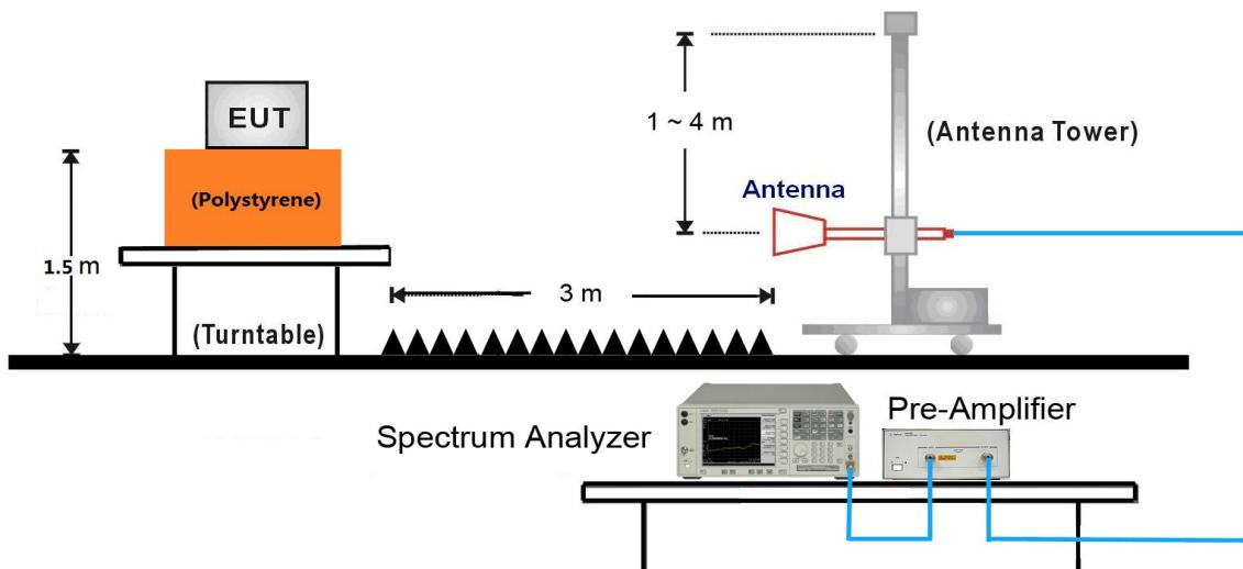
18GHz ~25GHz Test Setup:
