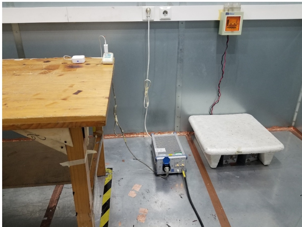
Picture 2: Conducted Emissions Test Setup
