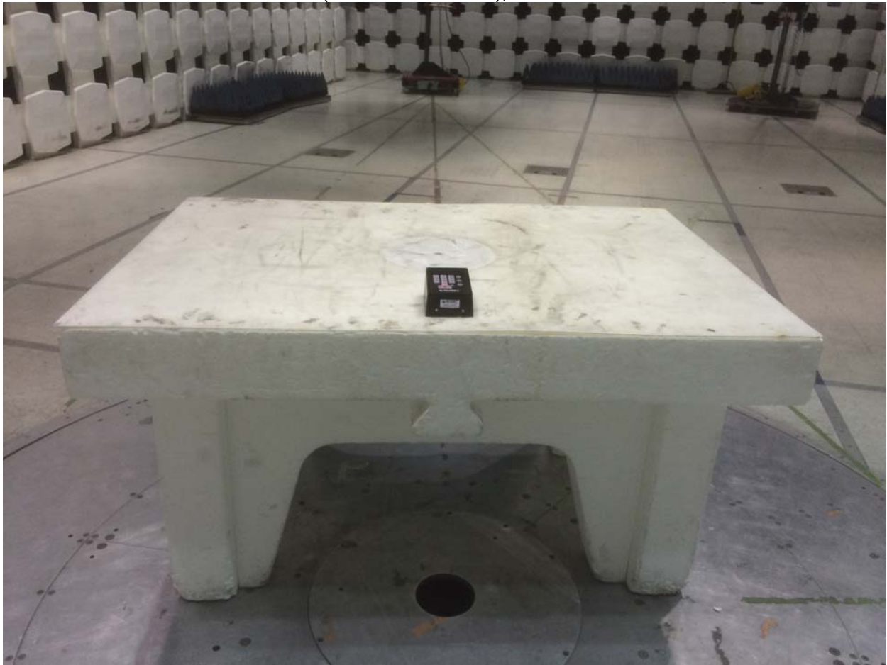
Z-axis (EUT sits on its back), 30-1000 MHz
