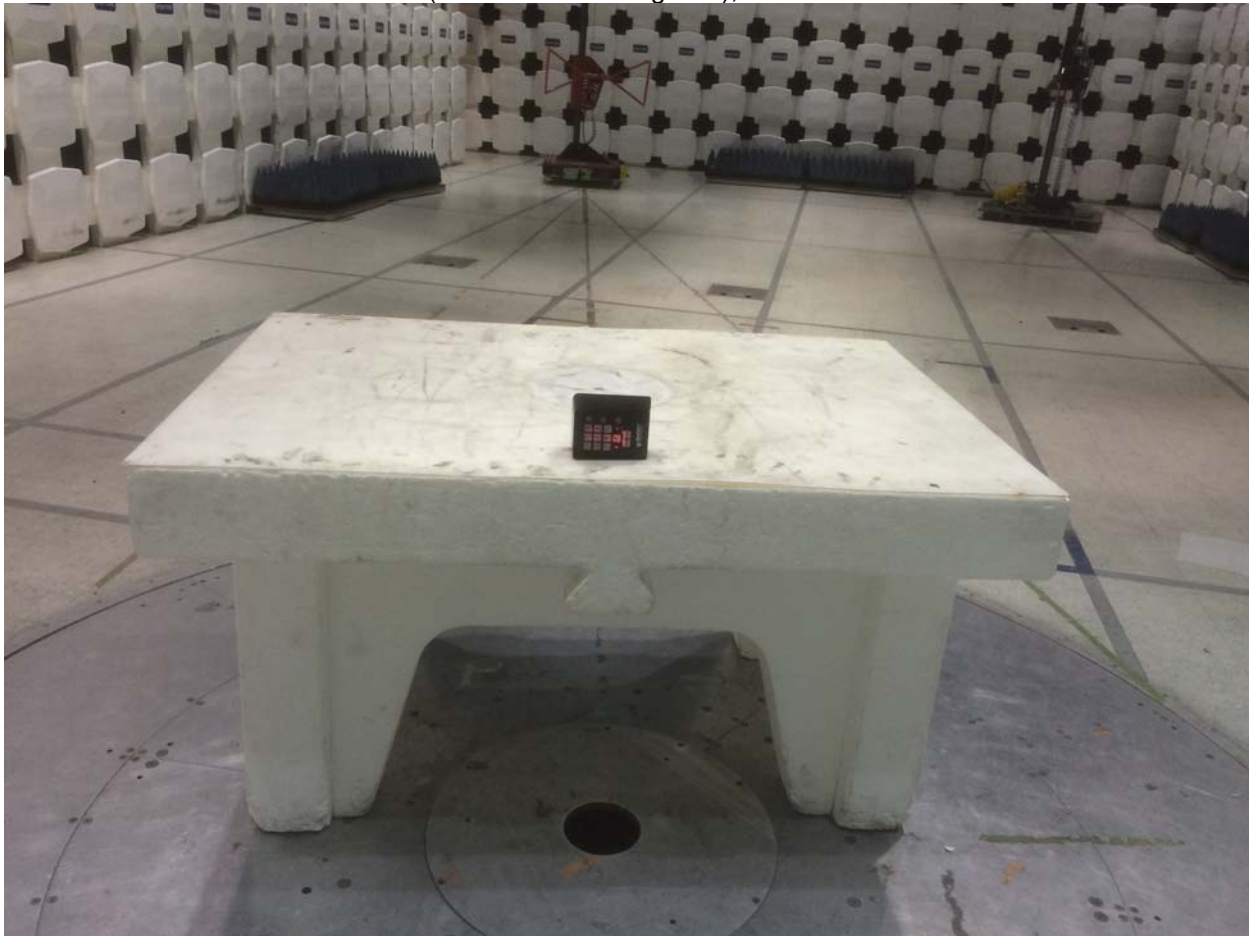
Y-axis (EUT sits on its long side), 30-1000 MHz
