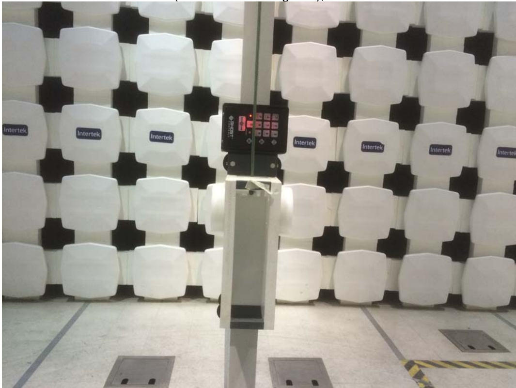
Y-axis (EUT sits on its long side), 1-4.5 GHz
