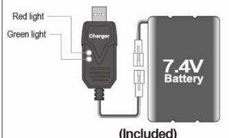
When charging the battery, the USB red light and green light will be flashing in the same time, the green light will keep eternal bright 'ON' and the red light will be OFF when finish charging.
