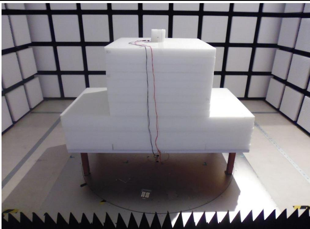
**Radiated Emission Above 1GHz Test**
