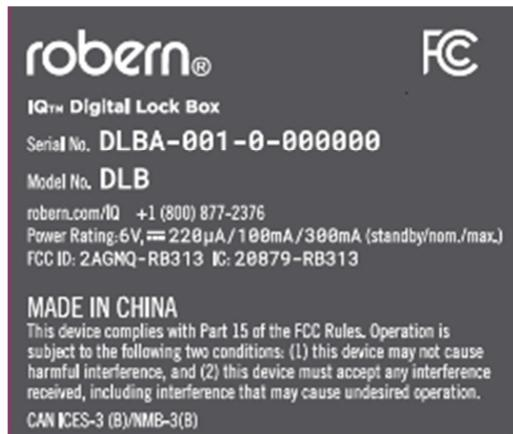
Specifications: The label shall be securely affixed to a permanently attached part of the device, in a location where it is visible or easily accessible to the user, and shall not be readily detachable. The label shall be sufficiently durable to remain fully legible and intact on the device in all normal conditions of use throughout the device's expected lifetime.
