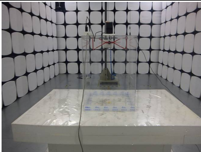
Radiated Spurious Emissions Test Setup Below 1GHz
