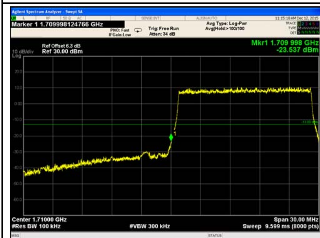
LTE Band 4 - Low Channel 16QAM-15
