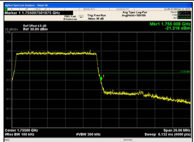
LTE Band 4 - High Channel 16QAM-10
