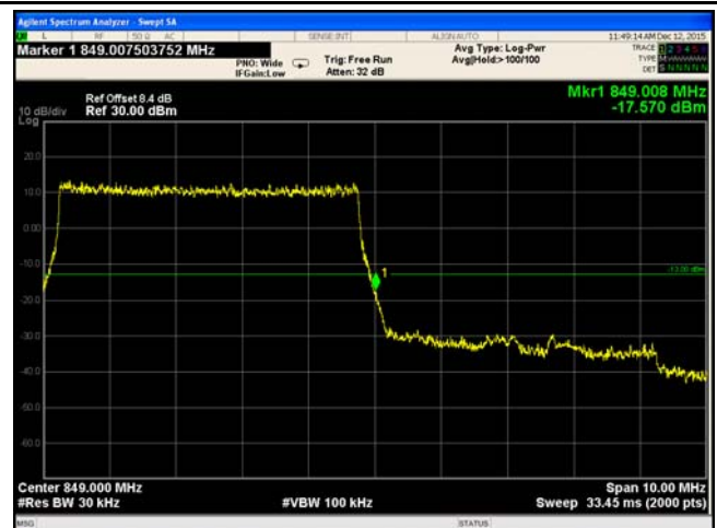
LTE Band 5 - High Channel QPSK-5
