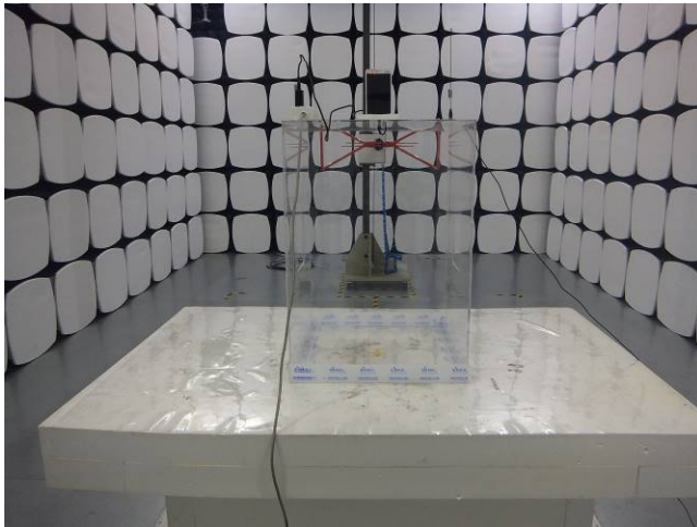
Radiated Spurious Emissions Test Setup Below 1GHz
