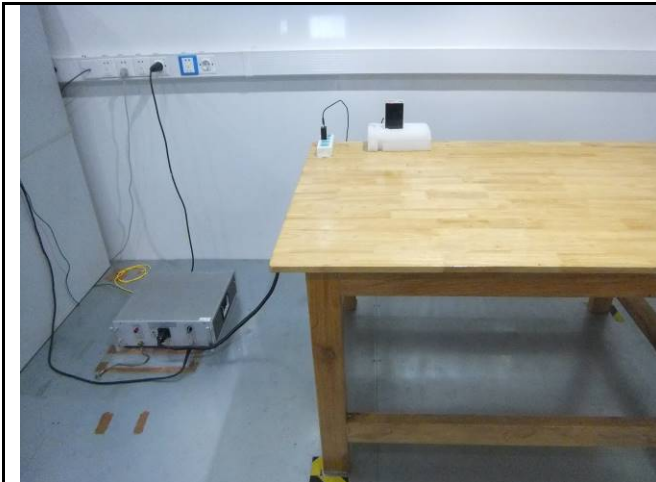
Conducted Emissions Test Setup Front View
