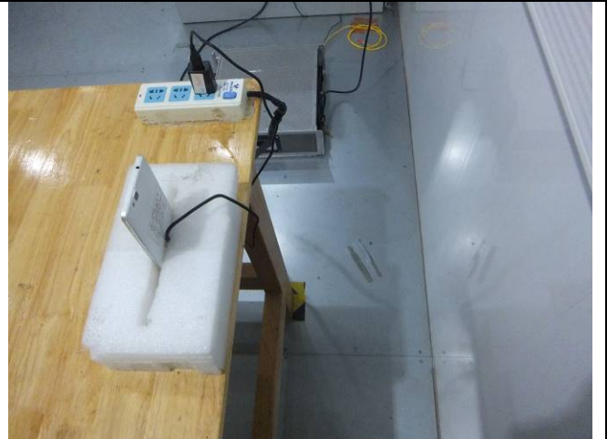
Conducted Emissions Test Setup Side View
