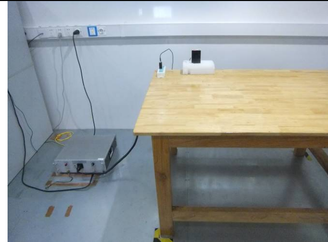
Conducted Emissions Test Setup Front View
