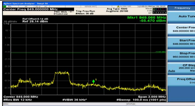
(Channel Bandwidth: 5 MHz)_HCH_QPSK_1RB#12
