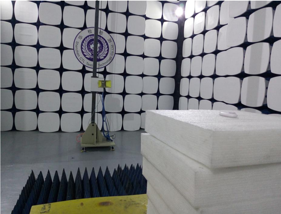
Above 1GHz: Test height 1.5m, the styrofoam block placed in the 0.8 m high test table
