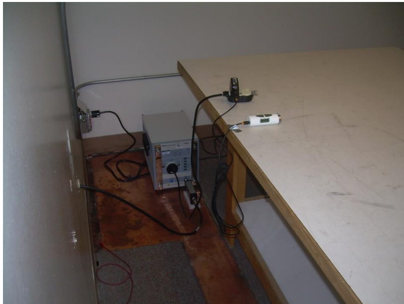
Photograph 7: Back View Conducted Emissions Worst Case Configuration
