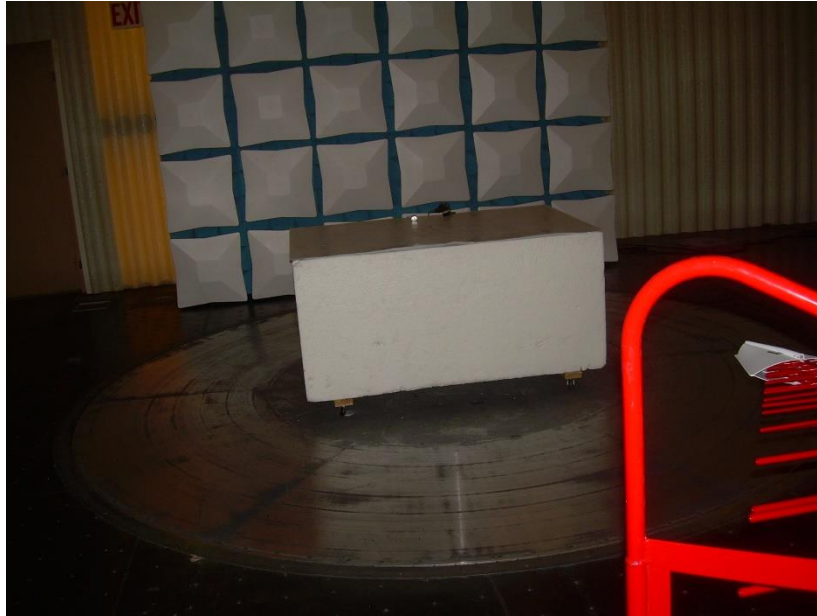
Photograph 1: Front View Radiated Emissions Worst Case Configuration
