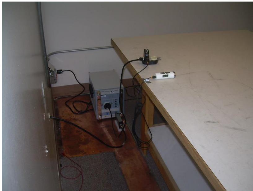
Photograph 6: Back View Conducted Emissions Worst-Case Configuration
