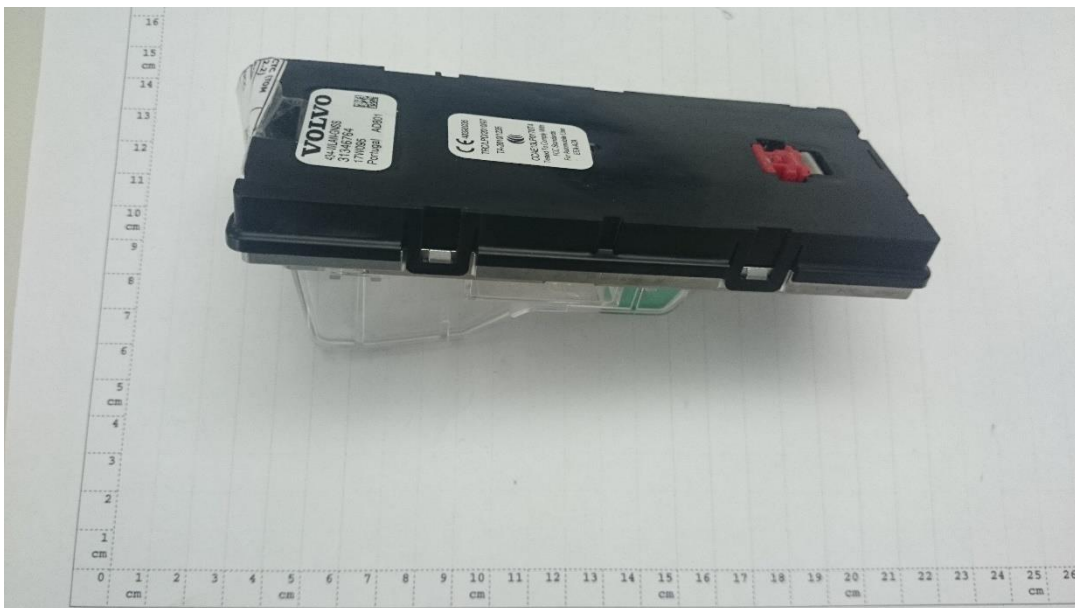
Photograph 12: Wifi antenna right side view
