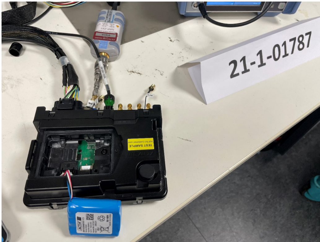
Fig. Mea.: 1 : Conducted measurement close up view
