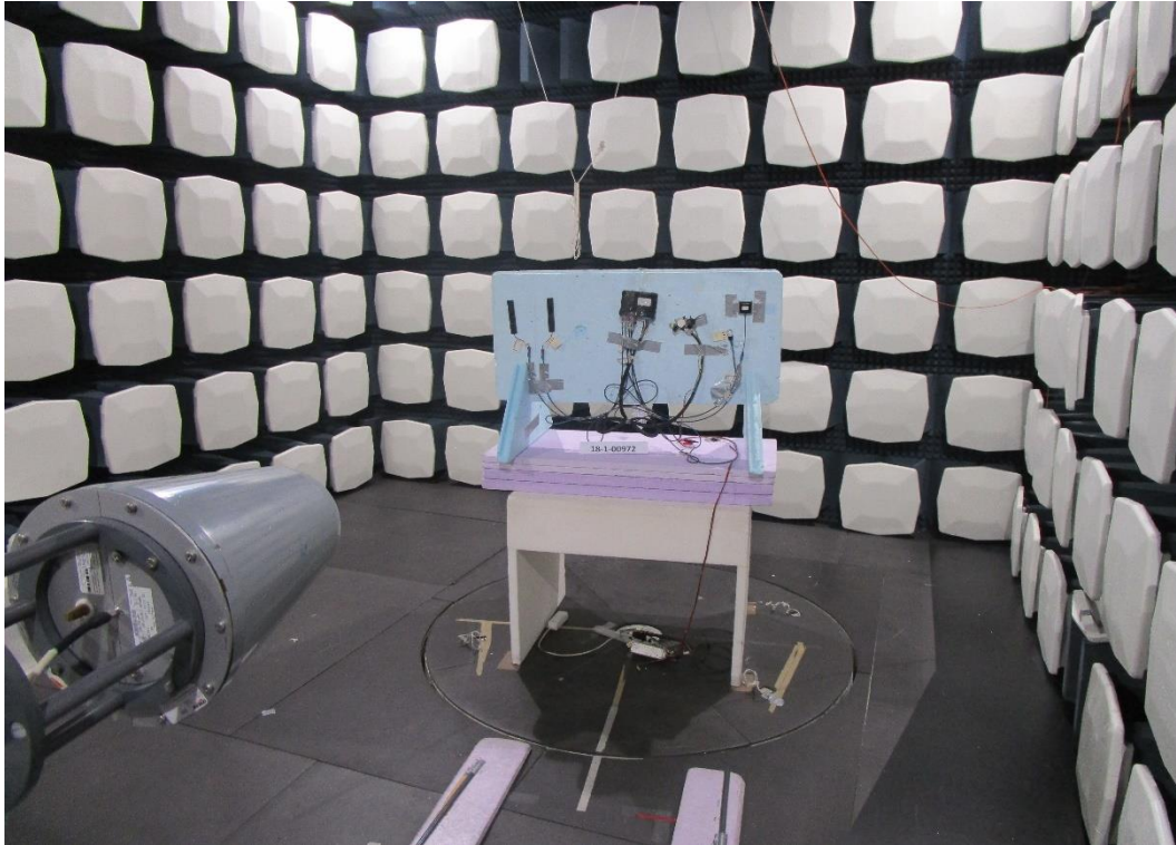
EUT setup overall view (EUT Position Standing)
