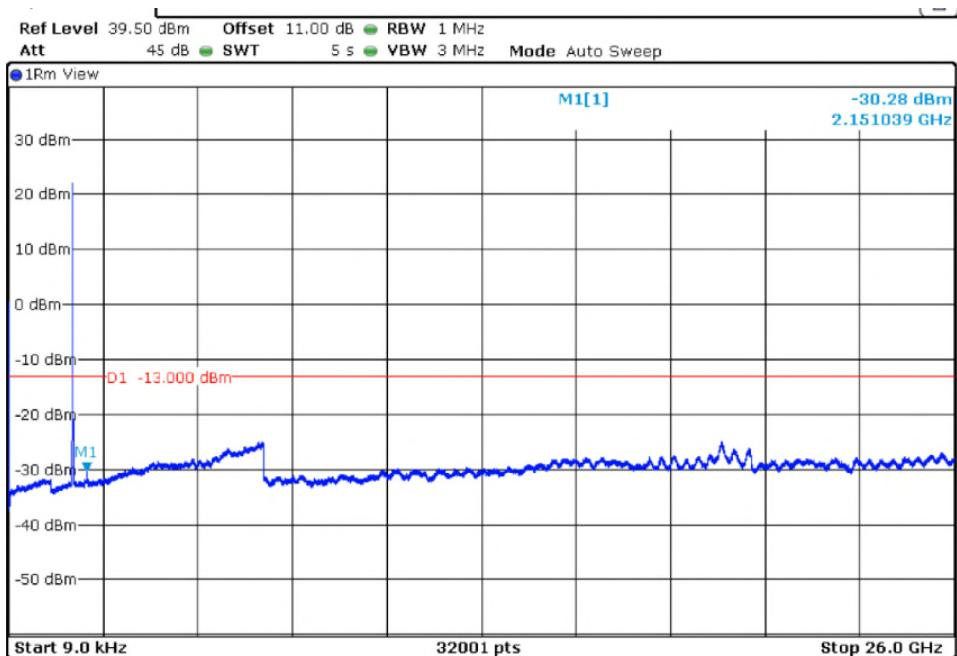
LTE QPSK MODULATION, BW = 20 MHz
