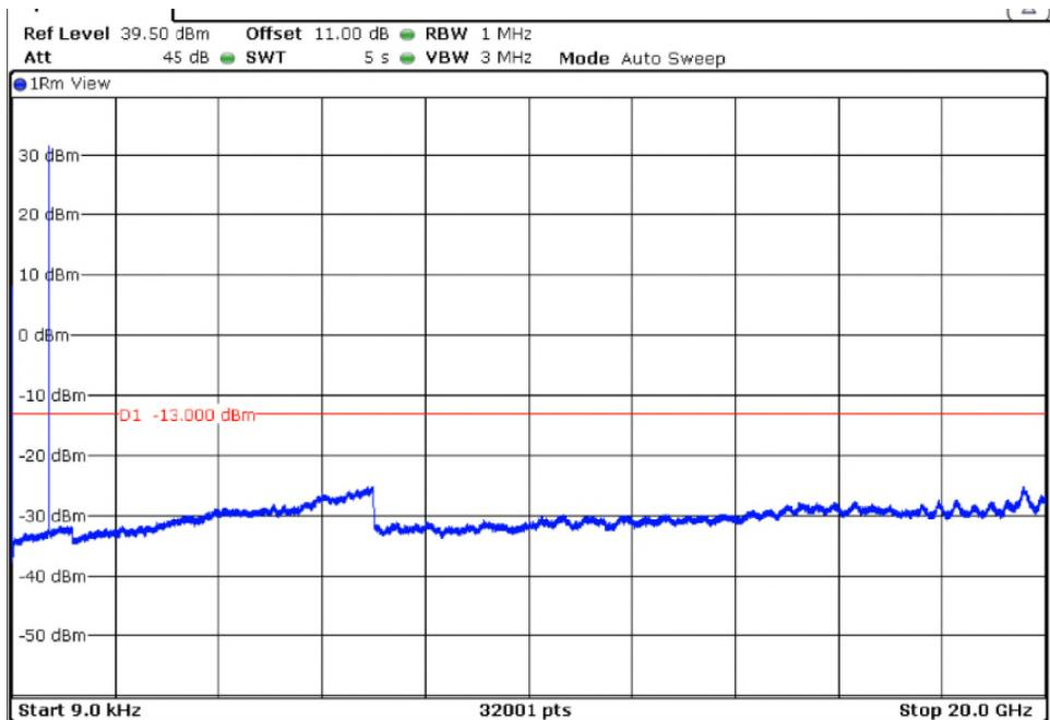
LTE QPSK MODULATION. BW = 3 MHz
