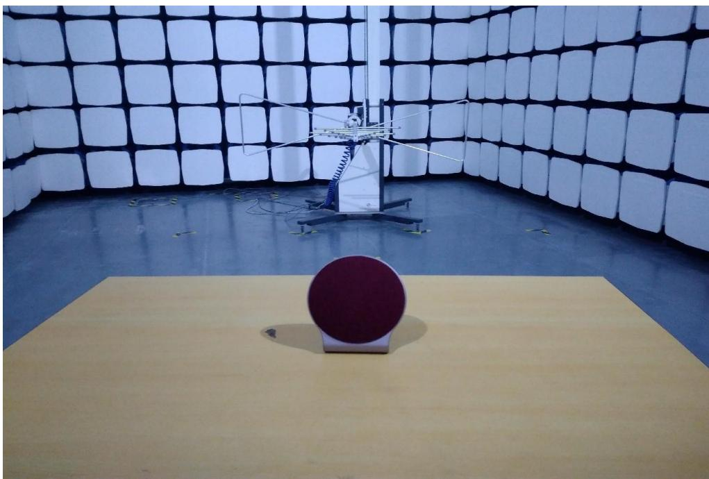
**Radiated Emission test view (Above 1GHz)**
