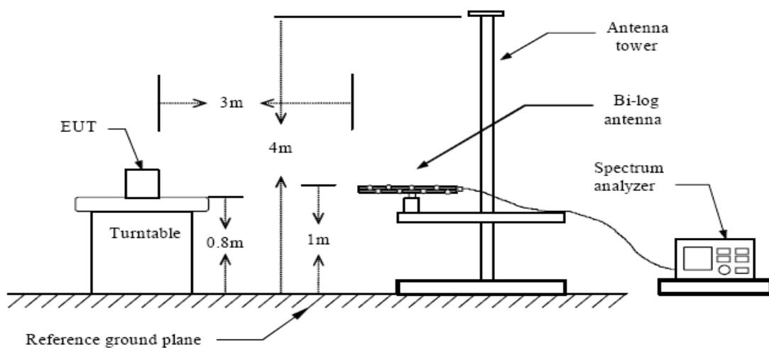
For radiated spurious emissions above 1GHz
