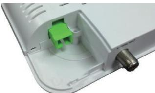
3.) Insert the fiber into the cover slot and slide the cover back onto the 72xx unit.
