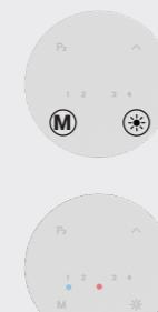
Both level & status LED indicator will turn on, the sensor enters detection status.
