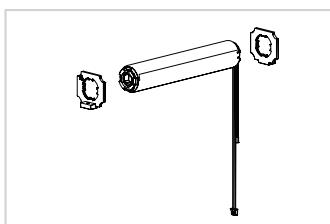
**Step 3.** Attach the shaft with adapter to the Motor assembly.
