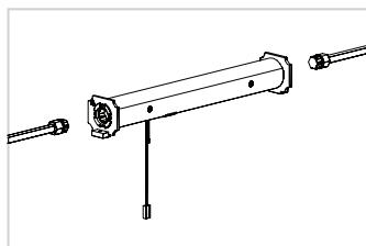
**Step 4.** Insert Motor assembly into the headrail.
