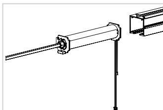
**Step 5.** Ensure power cord and antenna extend freely from the headrail. Anchor the Motor to the headrail.
