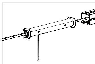
**Step 5.** Ensure power cord and antenna extend freely from the headrail. Anchor the Motor to the headrail where desired.
