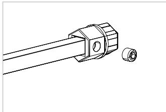
**Step 2.** Attach Headrail Adapters to the motor (2 each required).
