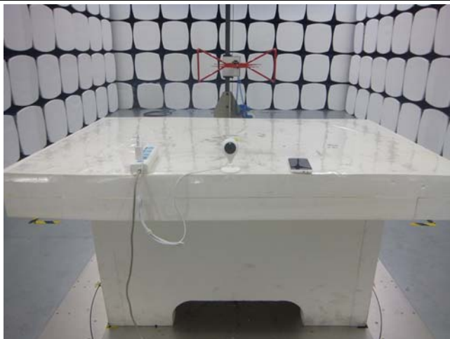
Conducted Emissions Test Setup Front View
