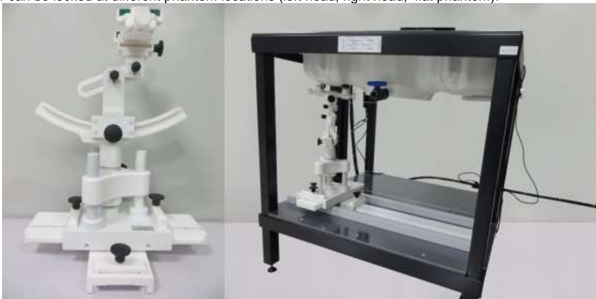
Device holder supplied by SATIMO
