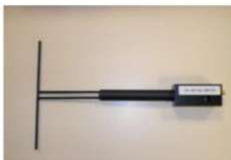
Figure 1 – Satimo COMOSAR Validation Dipole
