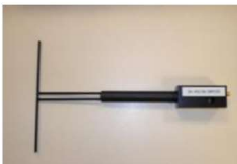
Figure 1 – Satimo COMOSAR Validation Dipole
