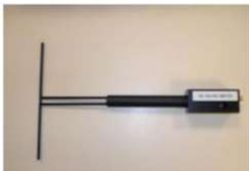
Figure 1 – Satimo COMOSAR Validation Dipole
