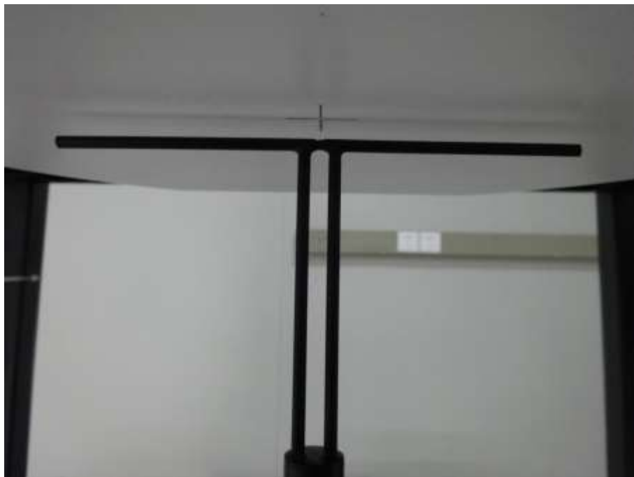
Photo of Dipole Setup
