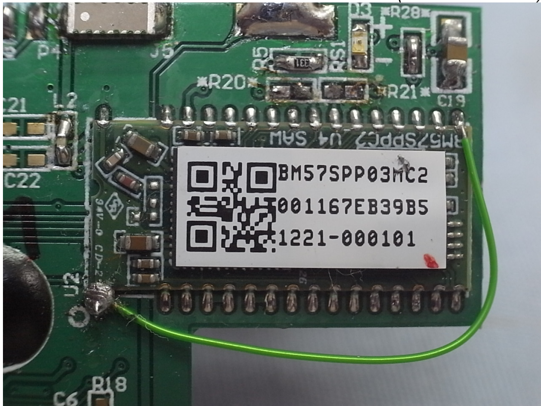
Figure 7 Internal View (RF Module Board)
