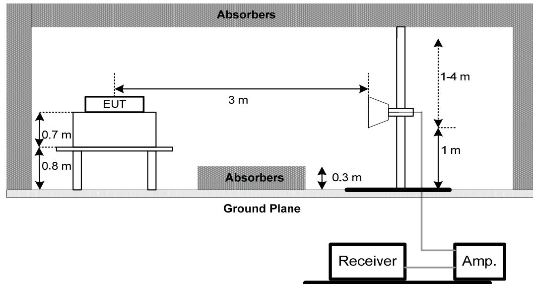
(C) For radiated emissions below 30MHz
