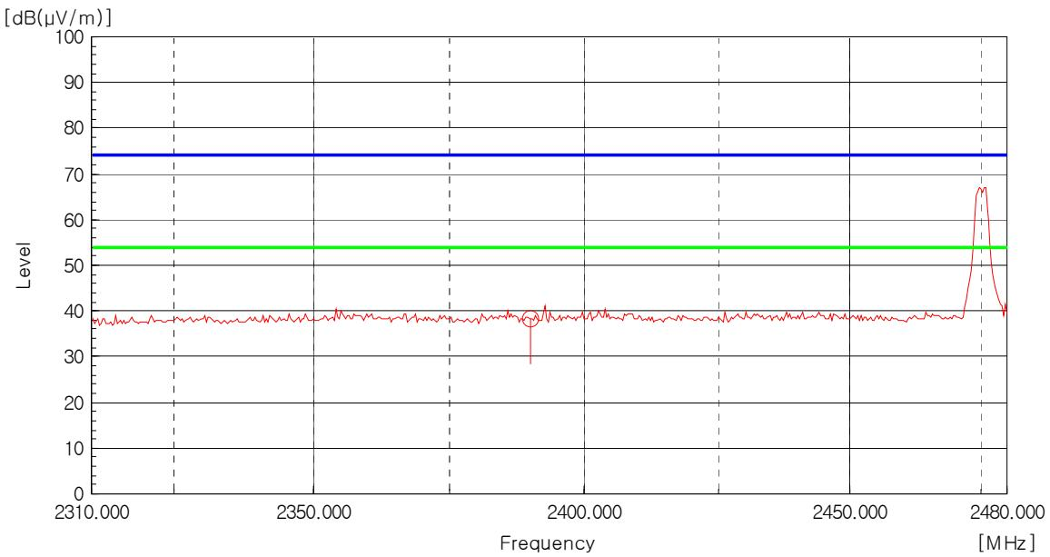
AV Detector: RBW: 1 MHz, VBW: 10 Hz (2 310 MHz - 2 390 MHz), Worst case (Low, Horizontal)
