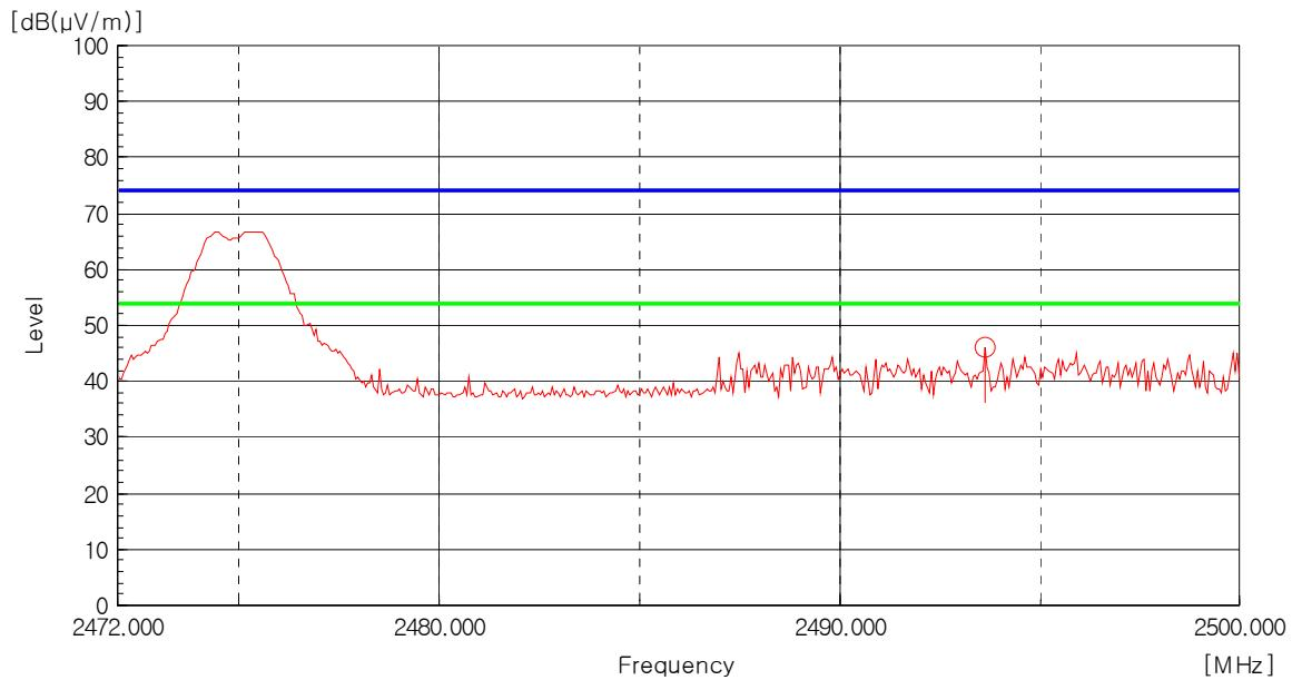
AV Detector: RBW: 1 MHz, VBW: 10 Hz (2 483.5 MHz - 2 500 MHz), Worst case (High, Horizontal)
