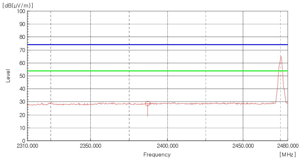
Peak Detector: RBW: 1 MHz, VBW: 1 MHz (2 483.5 MHz - 2 500 MHz), Worst case (High, Horizontal)
