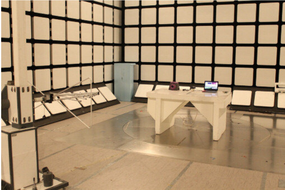
Photograph 5. The EUT and test set-up for radiated emission test (30MHz-1GHz).
