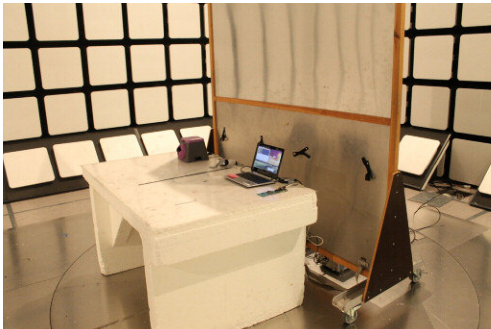
Photograph 4. The EUT and test set-up for conducted emission test.
