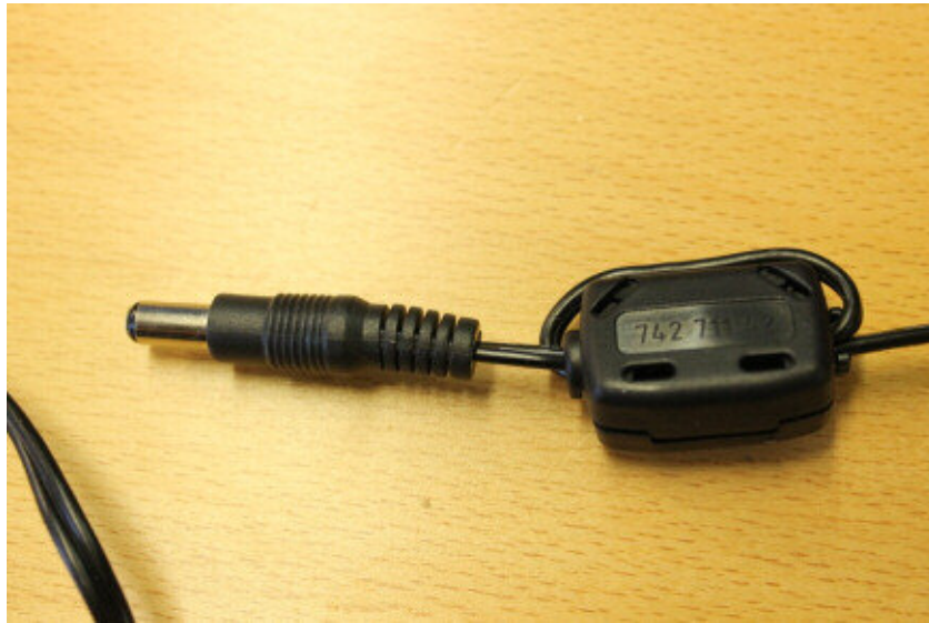
Photograph 3. Ferrite ring on the AC/DC converter cable (Würth Elektronik 742 711 42).
