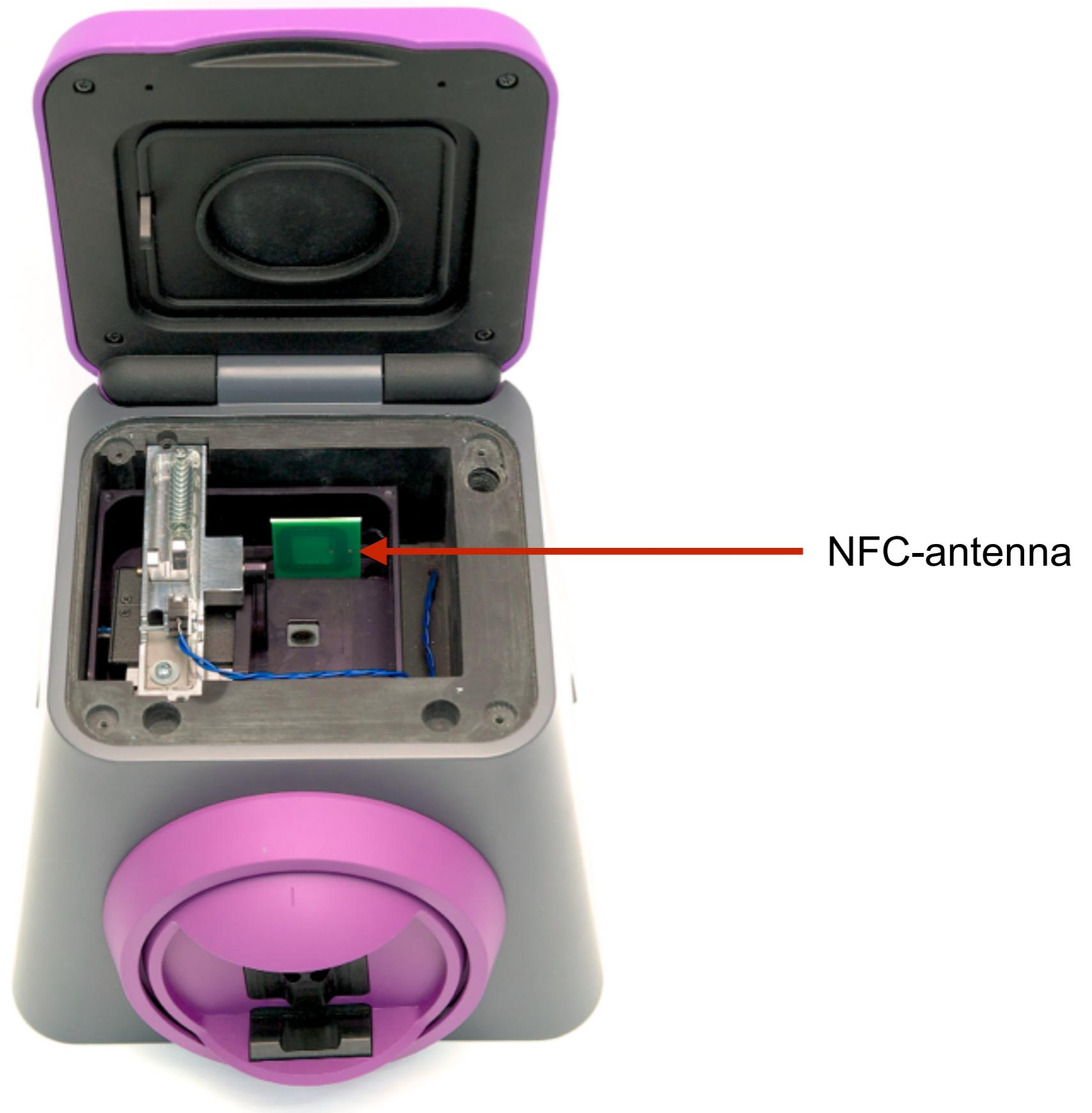
**Image 3. Lid opened, top cover removed, inner cover removed**
