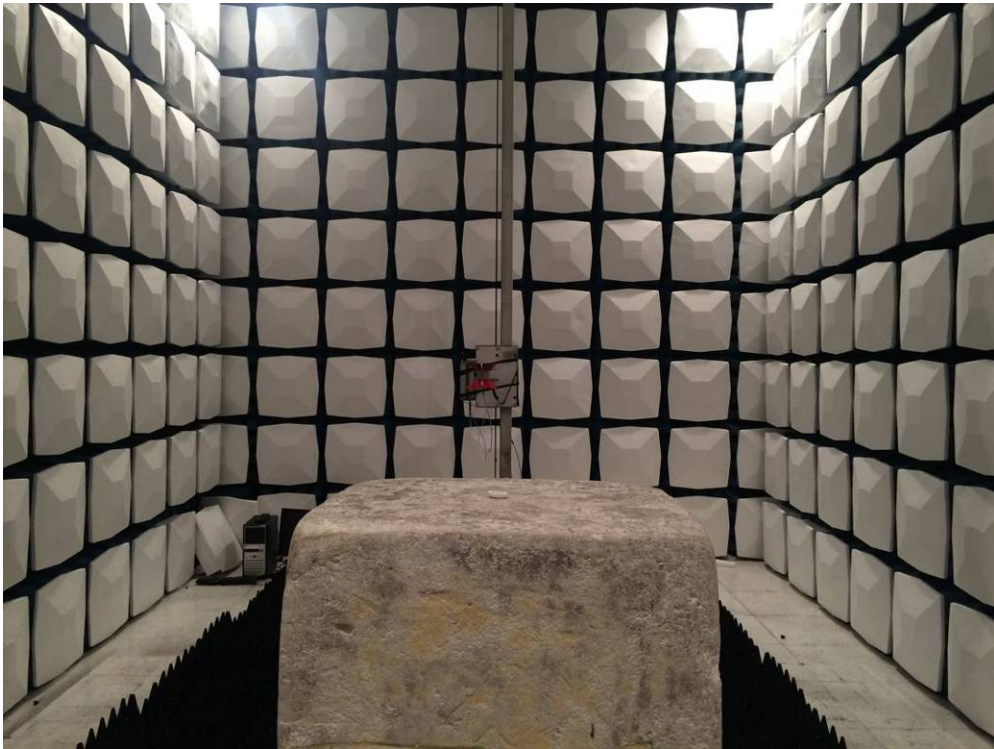
Description: Radiated Emission Test Setup for 1~18GHz
