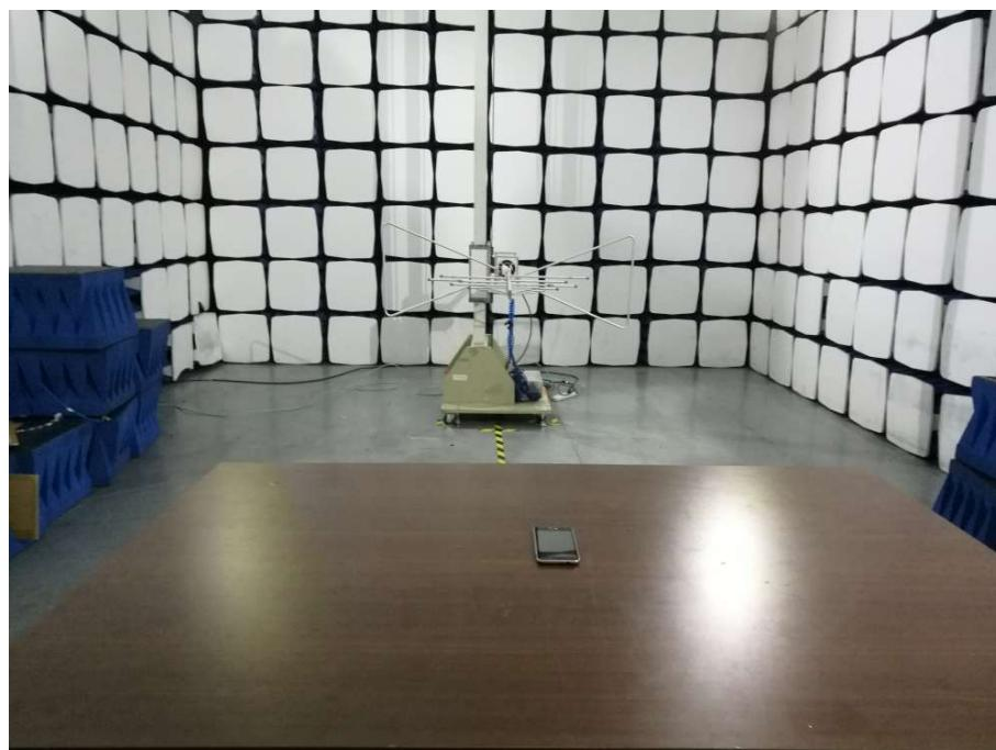
**Spurious Radiation Test Setup (1GHz to 18GHz)**
