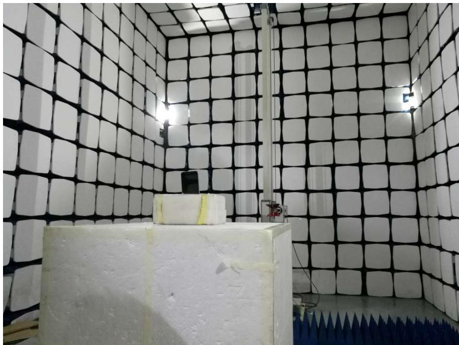
**Spurious Radiation Test Setup (Above 18G)**
