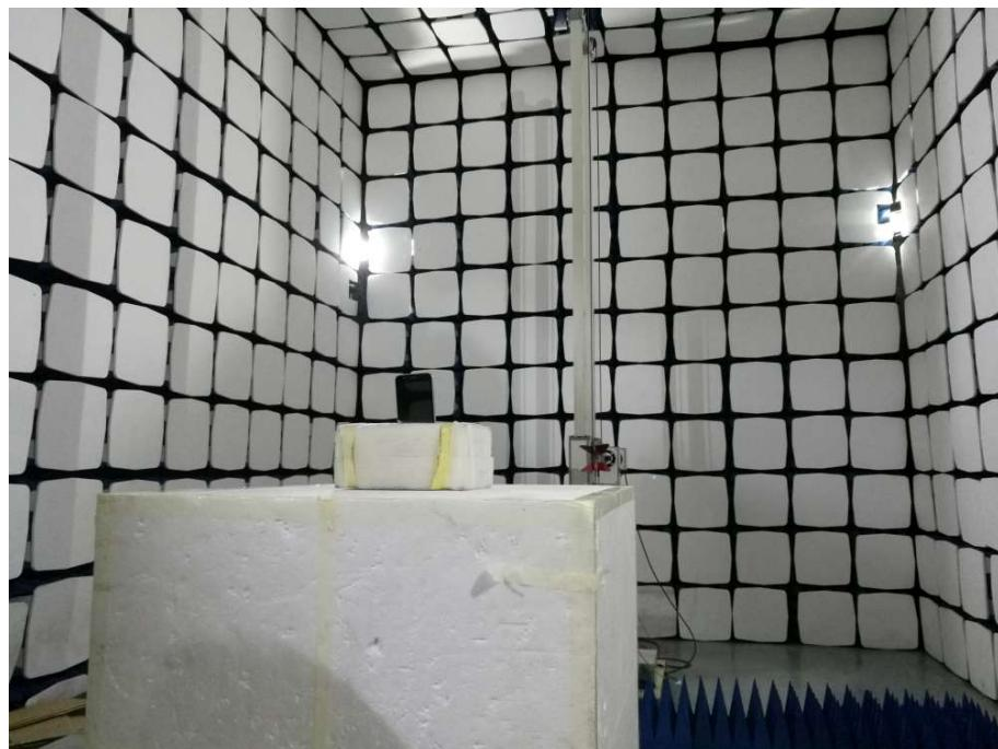
**Radiation Emission Test Setup (Above 18GHz)**
