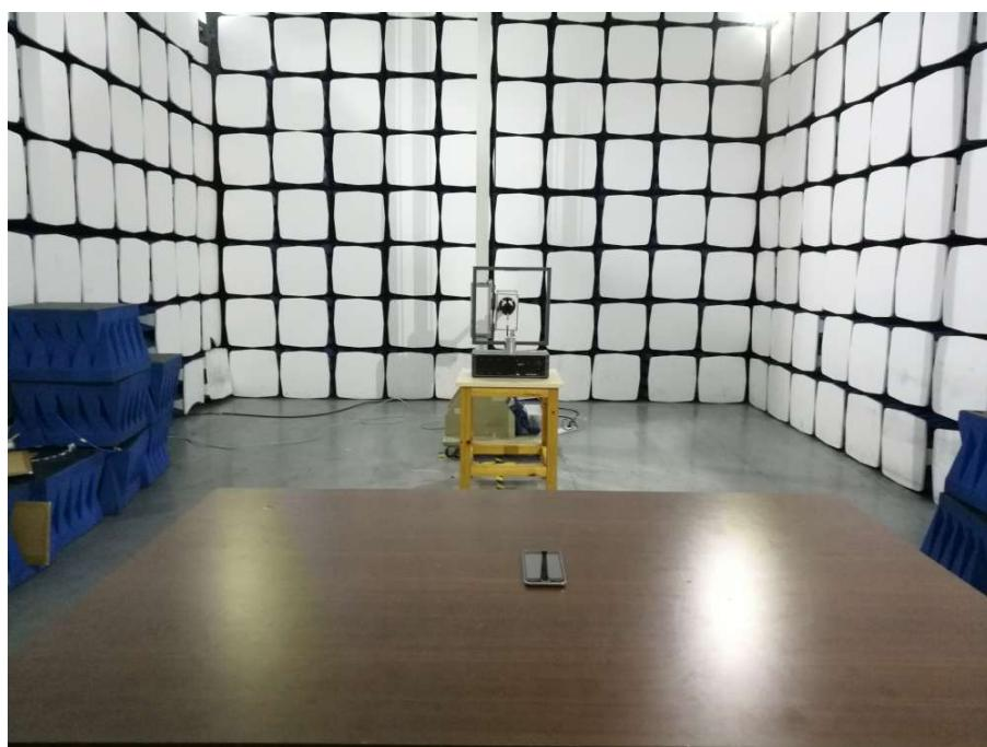
**Radiation Emission Test Setup (30MHz to 1GHz)**
