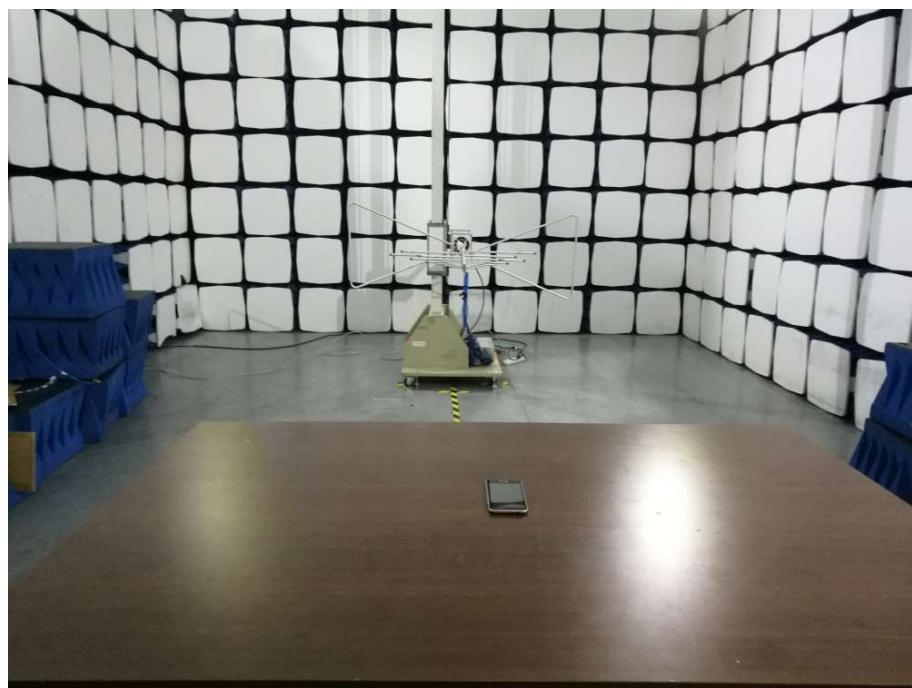
**Radiation Emission Test Setup (1GHz to 18GHz)**
