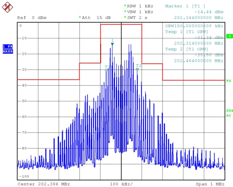
Emission Mask: input with 15 kHz AF, 50% modulation + 16dB.
