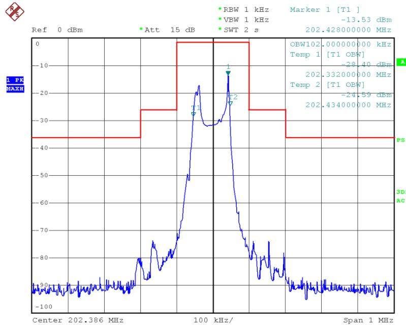
Emission Mask: input with 2500 Hz AF, 50% modulation + 16dB.
