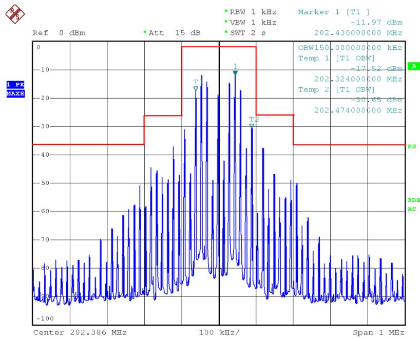
**Test results: The unit does meet the FCC requirements.**
