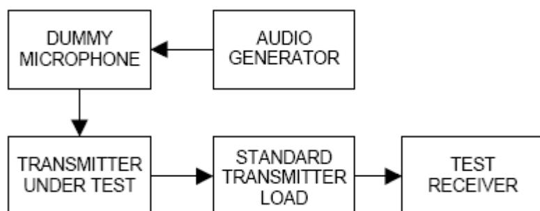
Input 2500Hz signal to the microphone, find the 50% rated deviation, add the level 16dB, test this status the 99% occupied bandwidth and record it.
