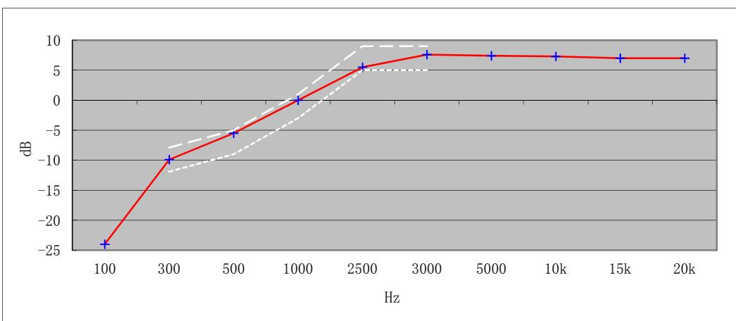
0dB=10mV at 1kHz (20% of the maximum rated system deviation).
