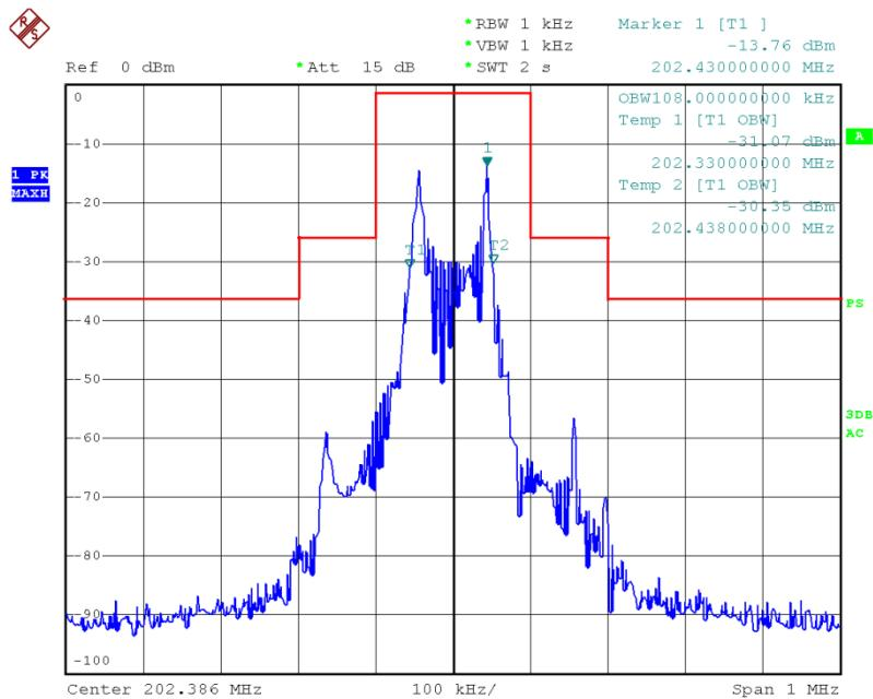
Emission Mask: input with 10 kHz AF, 50% modulation + 16dB.
