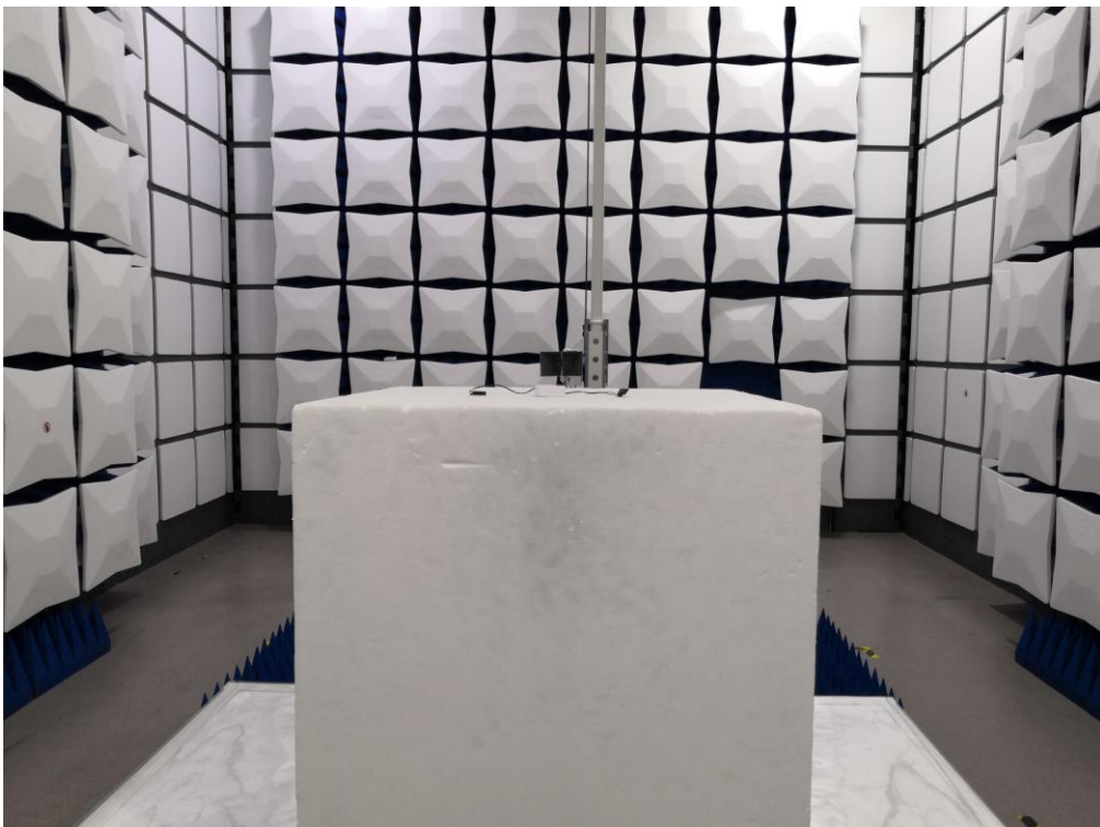
FCC RADIATED EMISSION TEST SETUP ABOVE 1GHZ
