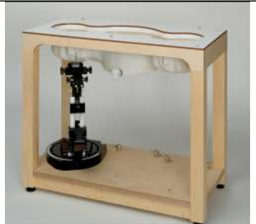
Fig. 8.7 Photo of SAM Twin Phantom
