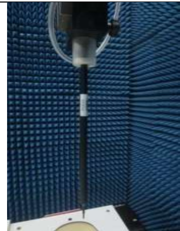
Fig. 8.2 Photo of E-Field Probe
