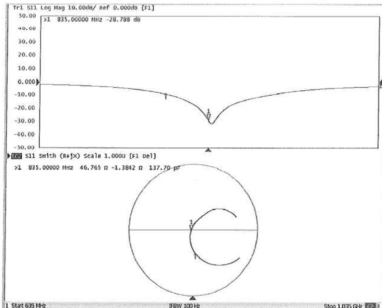
**D835V2,Serial No.4d114 Extended Dipole Calibrations**
