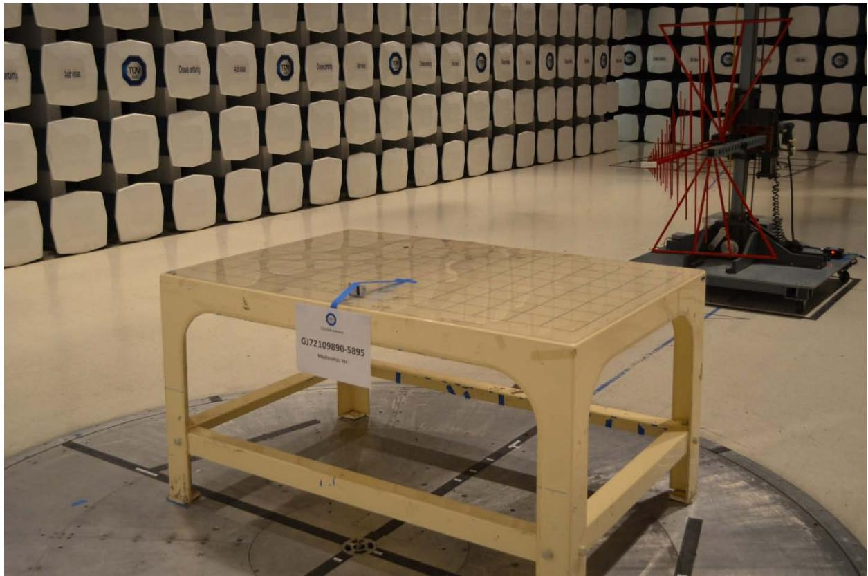
**Radiated Emissions Test Setup (below 1GHz Back)**
