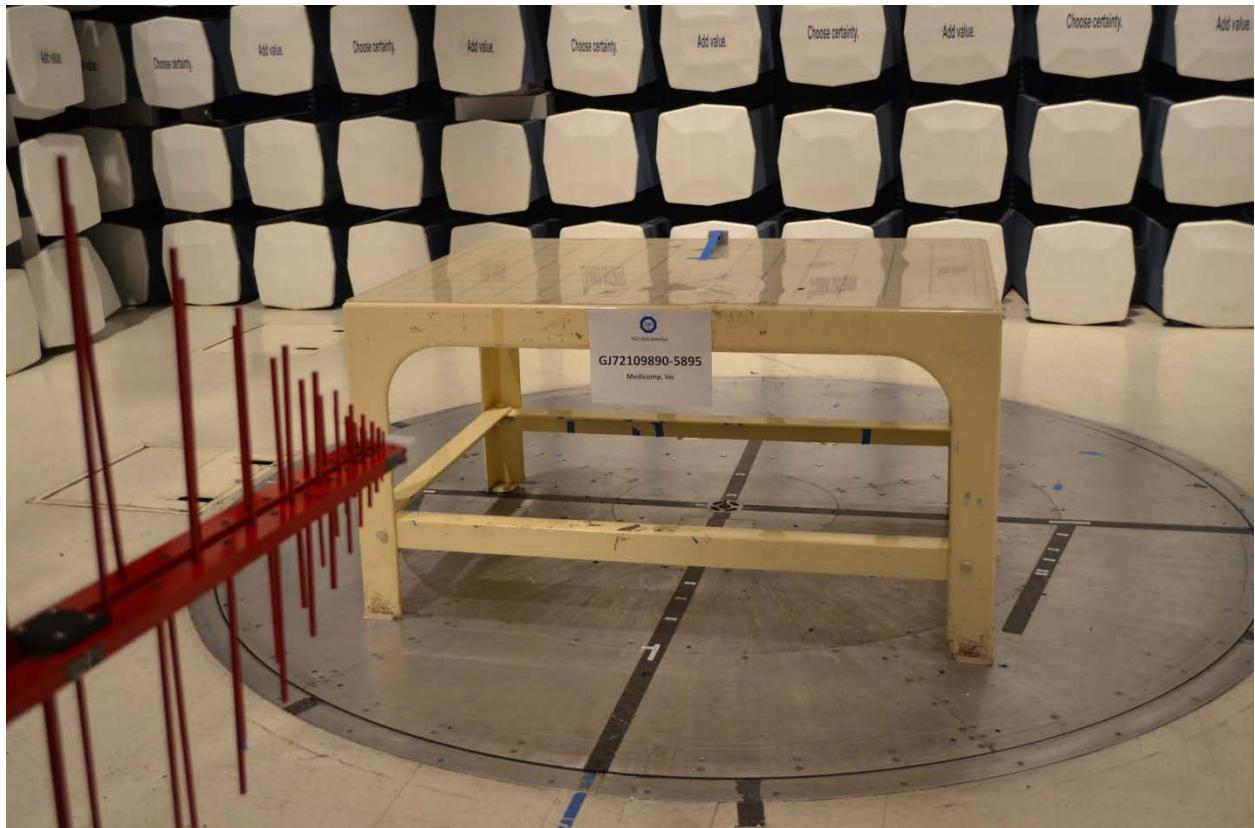
**Radiated Emissions Test Setup (below 1GHz Front)**
