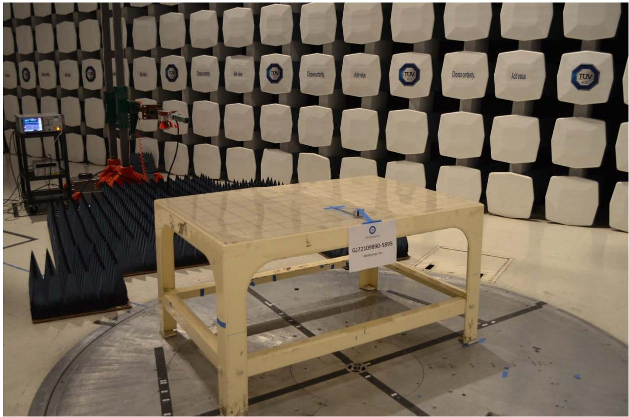
**Radiated Emissions Test Setup (above 1GHz Back)**
