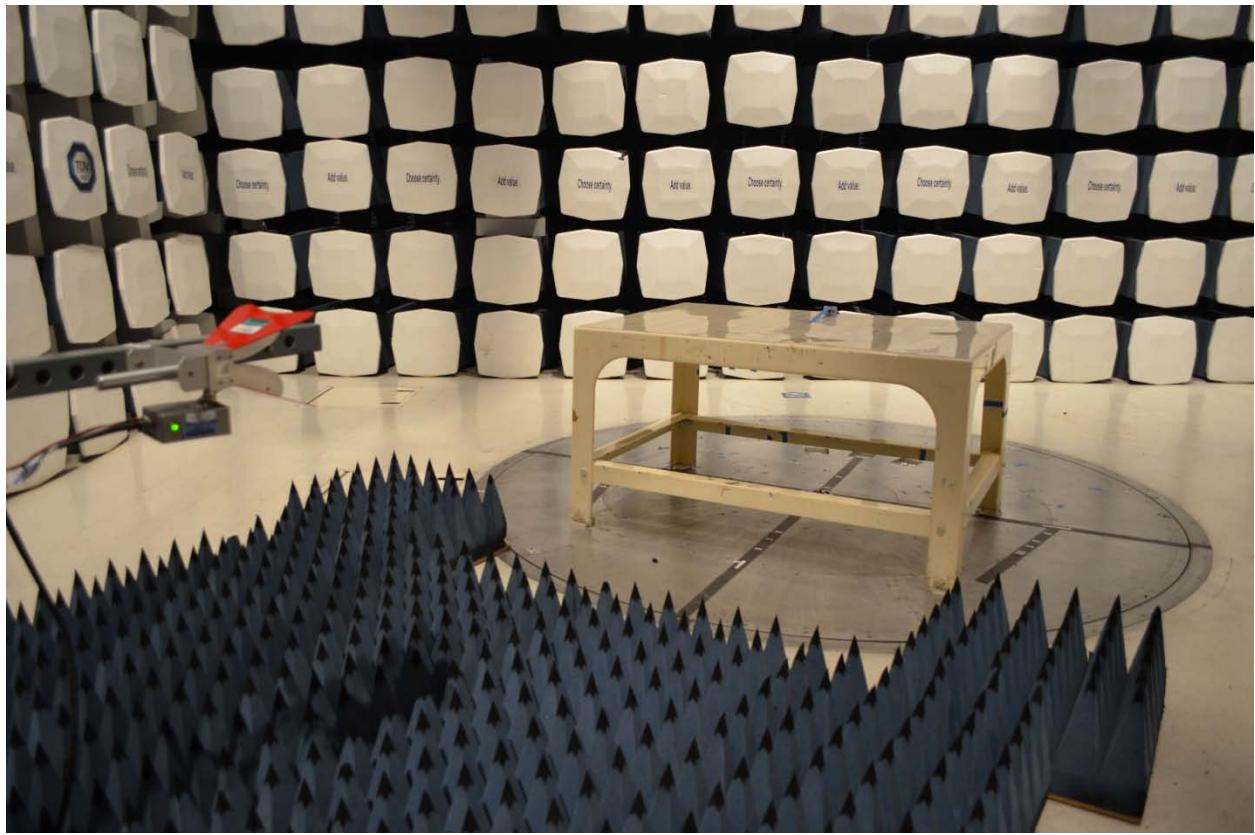
**Radiated Emissions Test Setup (above 1GHz Front)**
