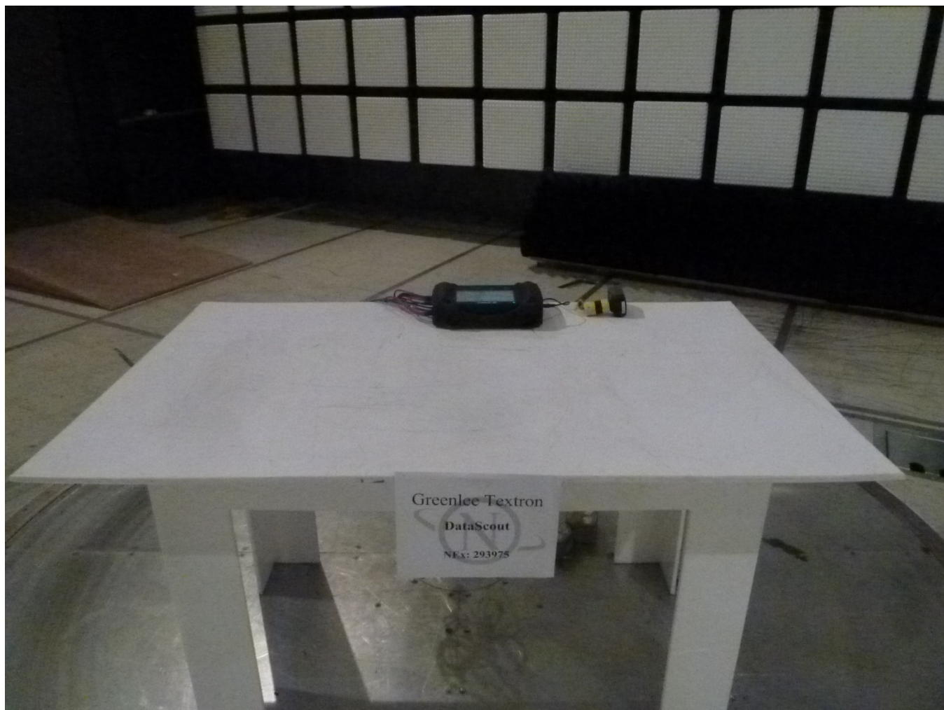
Figure 3.6-2: Setup Photo – Radiated Emissions < 1GHz
